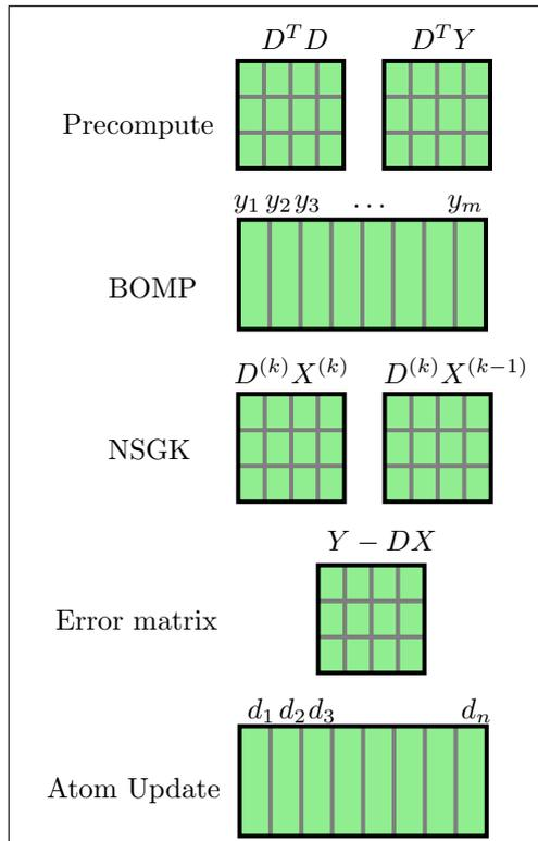
FIG. 1. Parallel DL: each row is executed simultaneously and each grid represents an OpenCL kernel whose elements are independent execution threads.
