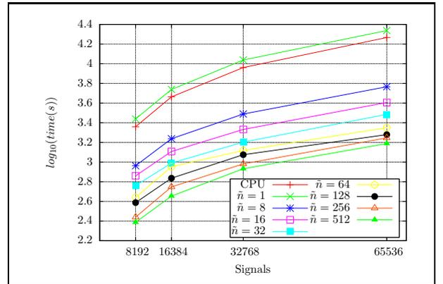
Fig. 3: Execution times for  $n = 512$ ,  $s = 8$ ,  $K = 100$ .
